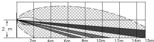
**Mouse 02 allows a range of 15 mt, the special lens shape provides a horizontal coverage of more than 90° with 29 patterns on 5 levels.**
