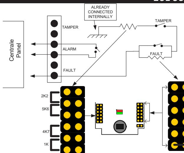
**ALARM = N.C. DOUBLE: FAULT - TAMPER**
