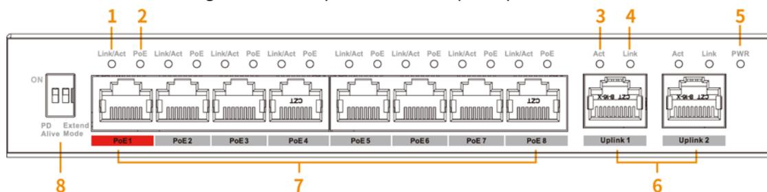
Following are all the ports and indicators on the front panel of the 4&8-port unmanaged desktop switch (without optical ports), and might differ from the actual product.
