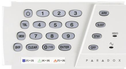
**IMPORTANT:** If installed on a partitioned system, the K636 will only display partition 1.
