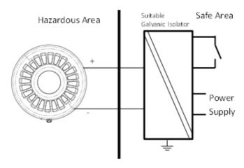
As with the Zener barriers, the second stage alarm can be triggered when using Galvanic Isolators, however an additional Intrinsically Safe relay is required to make the additional connection.
