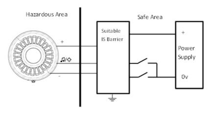
Switching between return paths for the 2 stage system will enable the 2nd tone. Second stage tone can be found in the table on page 12.
