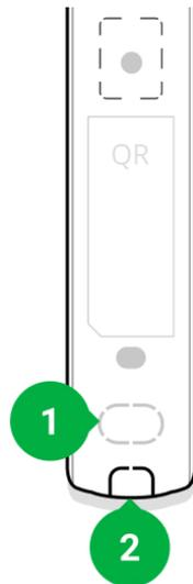
4. Run the cable from the hub into the detector enclosure through the hole made.
