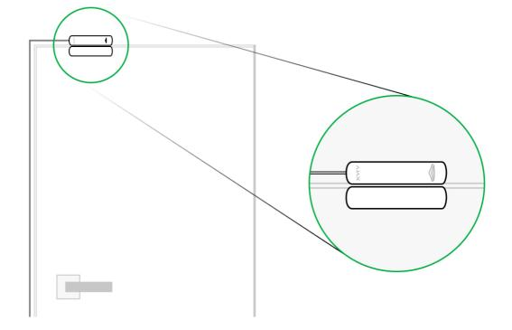
The sensitive element of the detector is a reed switch (**sealed contact**). This is a small flask with an open contact group inside. When a magnet is brought to the detector, a magnetic field is generated and the detector contacts are magnetized, attracted, and closed. Opening the flap or door moves the magnet away from the reed switch, which opens the circuit, and the detector detects opening.
