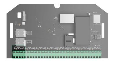
Hub Hybrid (2G) / (4G) has 8 Fibra lines. Numbers from 1 to 8 are indicated on the control panel board.
