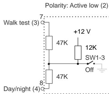
Walk test On = Pin 7 to GND
