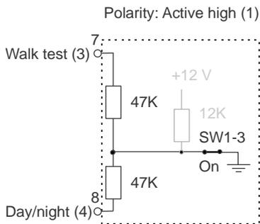
Walk test On = Pin 7 to +12 V
