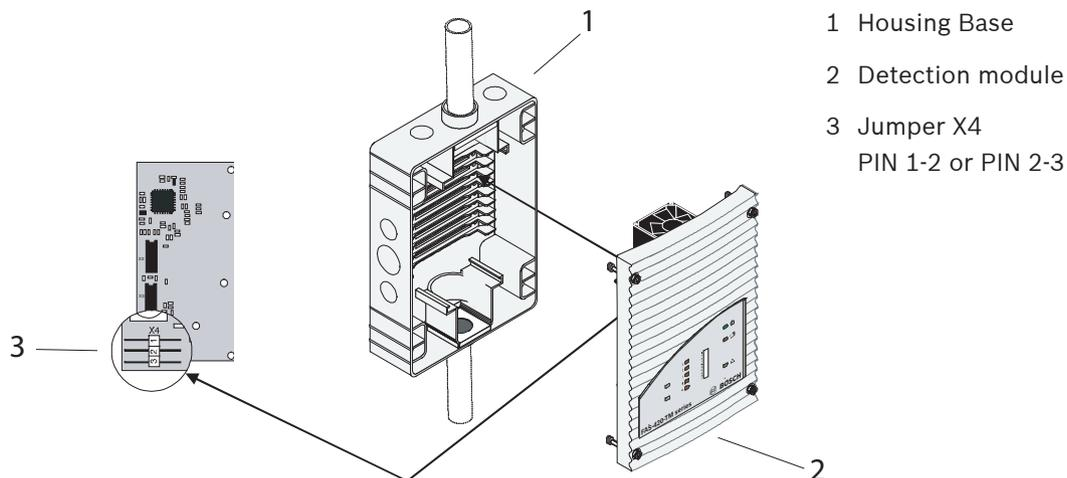
Inserting the detection module into the housing base
