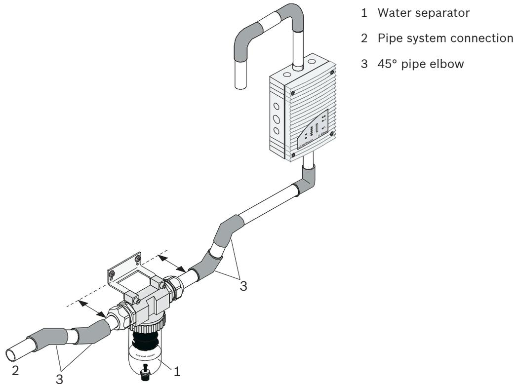
Installing the FAS-ASD-WS Water Separator in the pipe system
