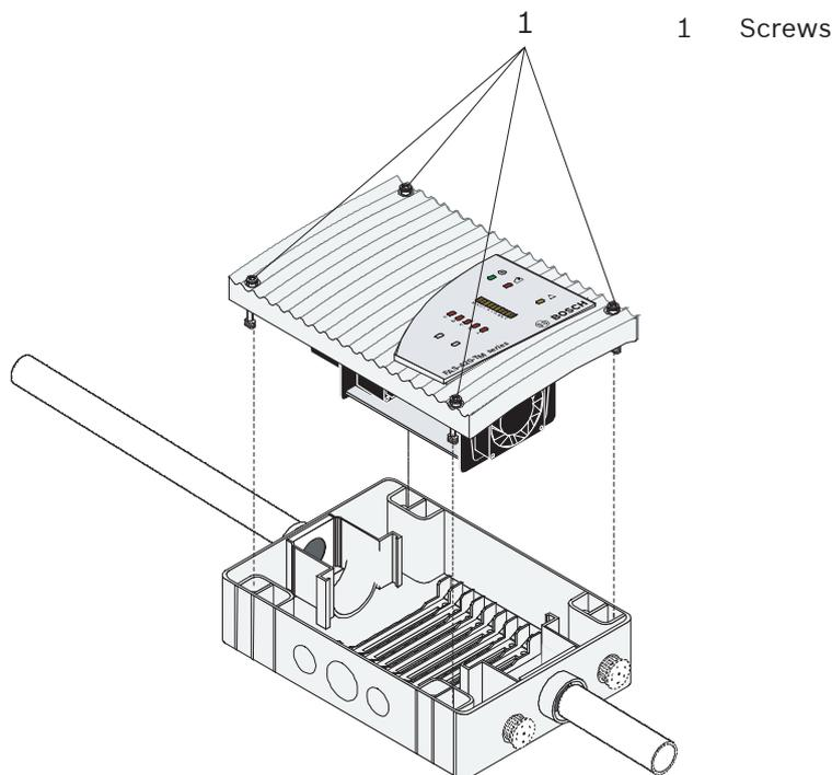
Replacing the detector module of the FAS-420-TM
