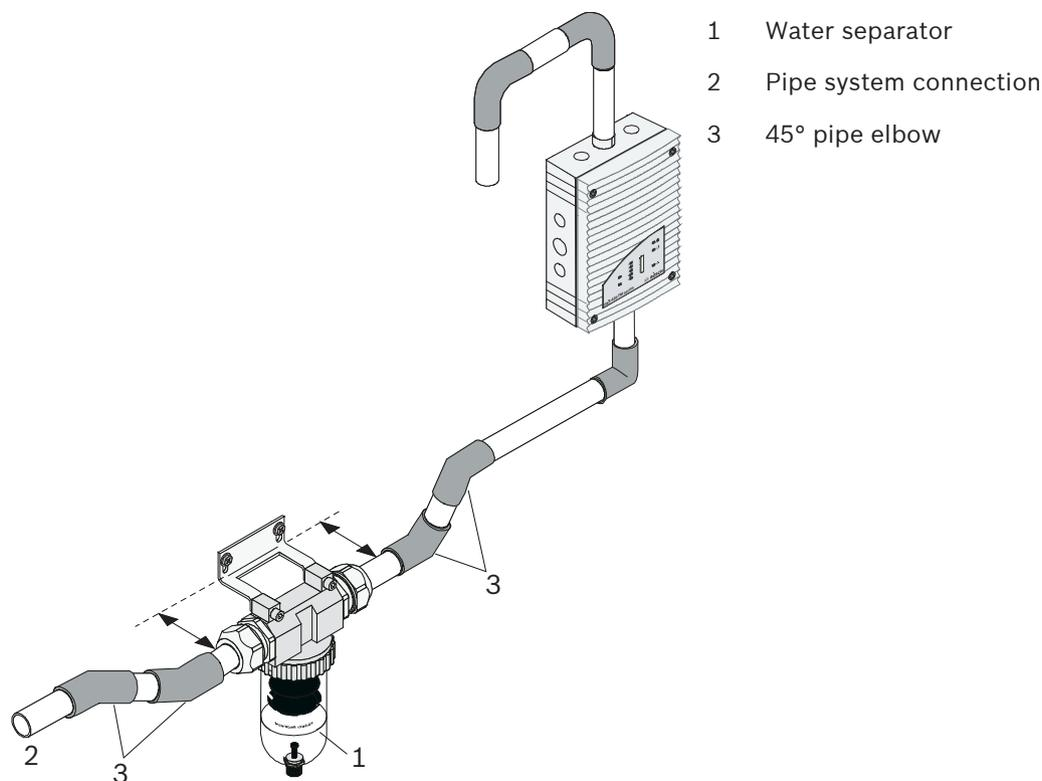
FAS-ASD-WS Water Separator for condensing water vapor and collecting condensate from the pipe system
