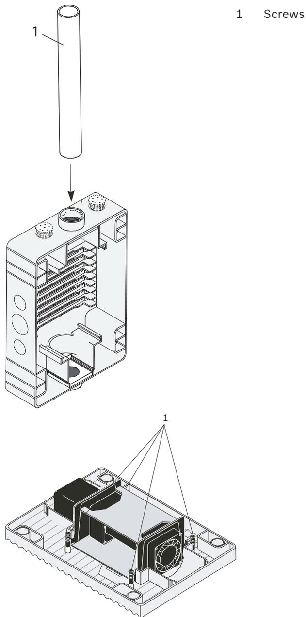
Turning the detection module in the cover of the FAS-420-TM detection unit
