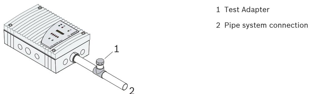
Installing the test adapter in the pipe system
