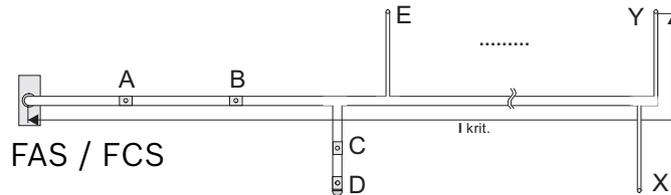
The branch pipes must be projected in accordance to the figure (project planning with branch pipes). The project planning of I-pipe described in the figure must be copied to every single sampling branch of other pipe forms (U, M, double-U pipe system).
