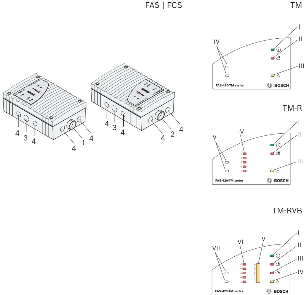
**Figure 3.5:** FAS-420-TM connections
