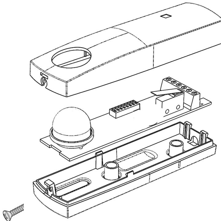
Fixed base rear slide the cable through the holes selected, secure the board in its housing interlocking and fix the cables into the appropriate terminals. Use the scrow to fix the top.
