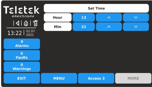
Use the up and down arrow buttons to set the time. You can also directly enter the new settings using the virtual digit keyboard after selecting the digit button for hour/minutes – item [4.1.3](#).
