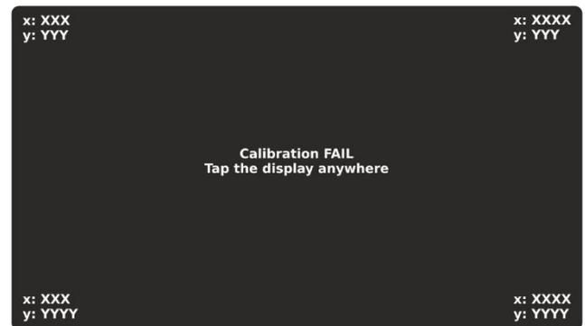
If the calibration is unsuccessful, it is announced with message for failure. In that case is recommended to perform the calibration again. Press the screen anywhere to return to DISPLAY menu.
