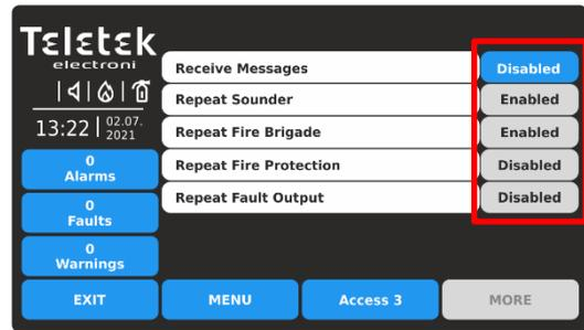
The receiving of messages for events is Disabled. The options for repeating the outputs status are unavailable for settings. *Even if there are options set as Enabled, they will be inactive and the panel will not repeat the status of any of the outputs.*
