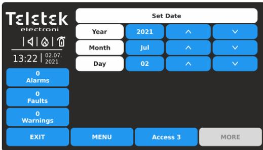
Use the up and down arrow buttons to set the date. You can also directly enter the new settings using the virtual keyboard after selecting the digit button for year/month/day – item [4.1.3](#). (Note: The months are entered with numbers – 1 for January, 2 for February, ... 11 – November and 12 for December.)
