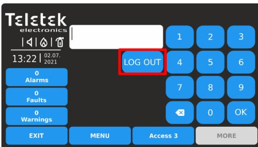
Press ACCESS button for changing the user Level. Press LOG OUT button for quick logging out.
