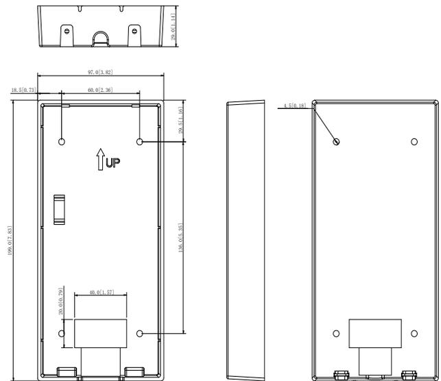
**Step 1** Drill screw holes in the wall according to the position of the screw holes in the mounting box, and then put the expansion tubes in the screw holes.
