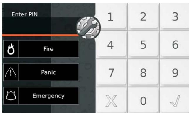
**Figure 25** Default labels of the Super Keys on the Touchscreen Keypad.
