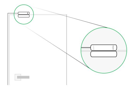
The sensitive element of the detector is a reed switch (**sealed contact**). This is a small flask with an open contact group inside. When a magnet is brought to the detector, a magnetic field is generated and the detector contacts are magnetized, attracted, and closed. Opening the flap or door moves the magnet away from the reed switch, which opens the circuit, and the detector detects opening.
