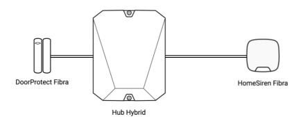
DoorProtect Fibra is a wired opening detector. The detector is connected to the hub via a wired bus and operates using the Fibra protocol. In case of standard installation, it consists of two blocks: a detector and a magnet. The detector is mounted on a frame or fixed part of the structure, and the magnet is mounted on a movable flap or a sliding part.
