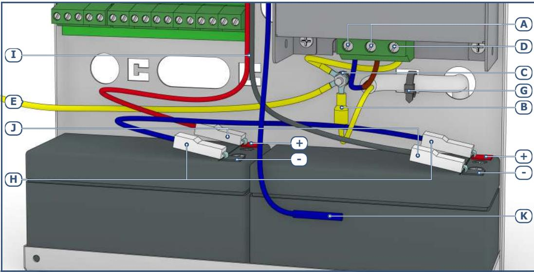
1. Connect the mains power supply to the terminals on the power-supply module ([A], table 1, K).
