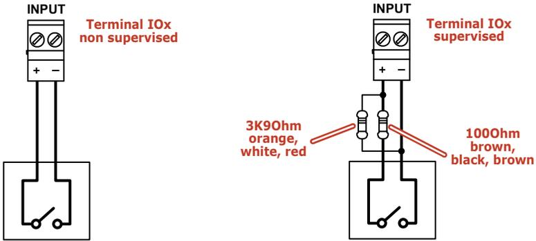
When supervision is enabled, the occurrence of open and short-circuit conditions will generate an "Interconnection fault".
