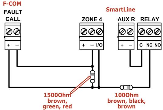
For SmartLine control panels it is necessary to enable the "Output to fault warning routing equipment" option using SmartLeague software, above version 3.5.1.6.
