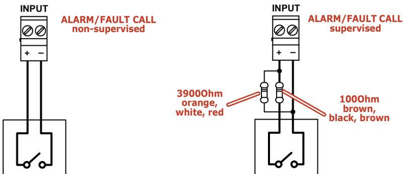
Following is the connection of the communicator with a SmartLine fire-detection control panel manufactured by Inim Electronics, for alarm and fault communications:
