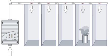
Figure 3.3: Phase 3: Blowing out
