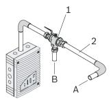
Components of manual blowing-out systems
