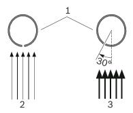
Positioning the air sampling opening depending on air speed
