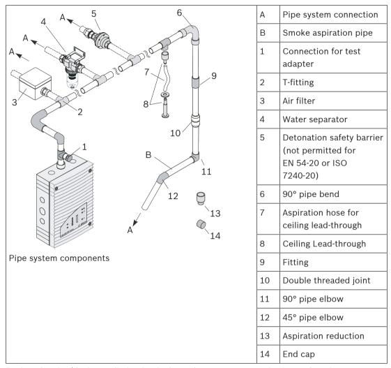
During planning/design, a distinction is drawn between area monitoring and equipment monitoring. For both applications, PVC pipes and halogen-free pipes can be used but the restrictions of EN 54.20 must be observed. The pipes used for equipment monitoring should be halogen-free.
