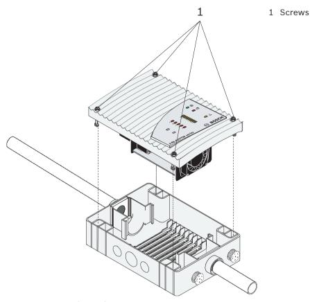
Replacing the air filter of the FAS-420-TM
