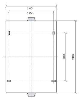
Figure 5.2: Bore distances of FAS-420-TM housing base
