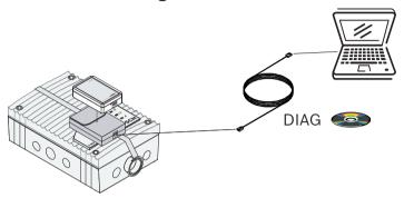
Figure 3.6: Diagnostic software for importing and reading out the device data
