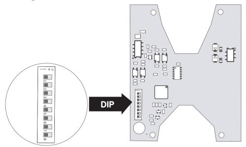
Figure 5.1: Setting the detector address
