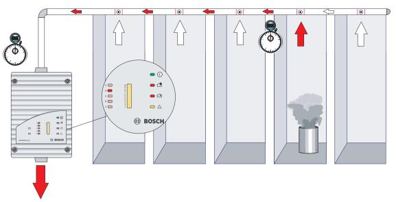
Figure 3.4: Phase 4: Identification of fire source by reversing the fan's direction of flow
