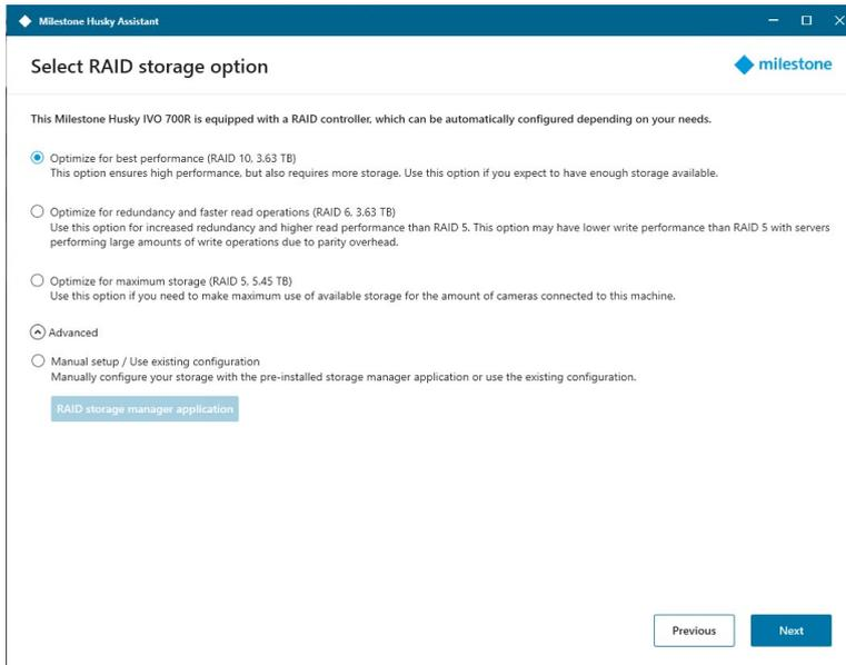
The **Advanced** option is to manually configure the RAID using the RAID storage manager application.
