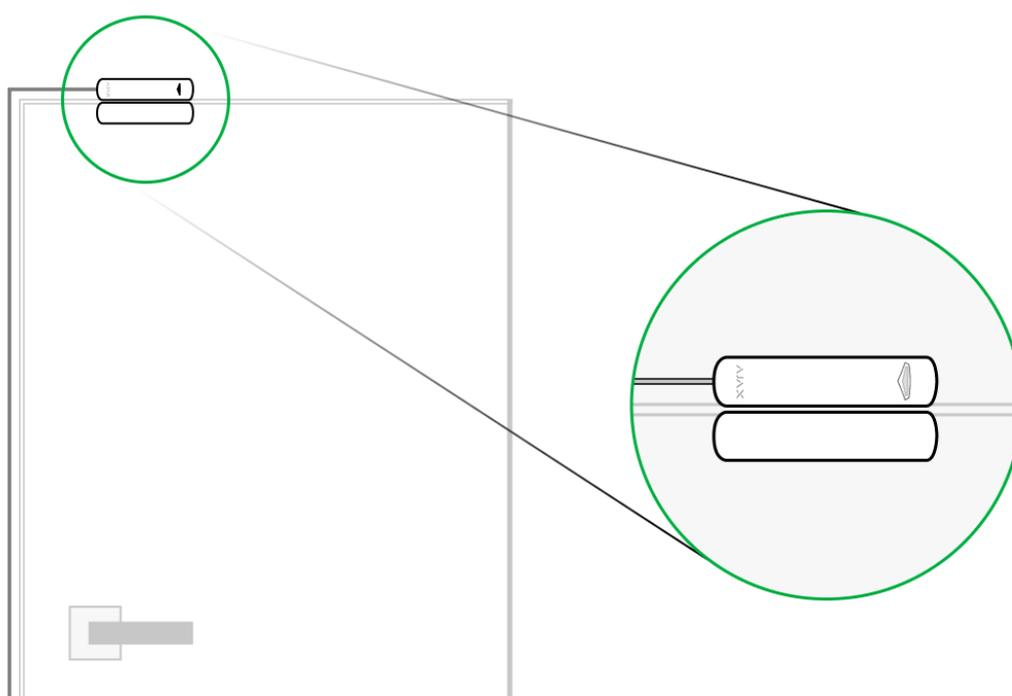
The sensitive element of the detector is a reed switch (**sealed contact**). This is a small flask with an open contact group inside. When a magnet is brought to the detector, a magnetic field is generated and the detector contacts are magnetized, attracted, and closed. Opening the flap or door moves the magnet away from the reed switch, which opens the circuit, and the detector detects opening.
