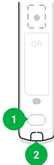
4. Route the cable from the hub into the detector enclosure through the hole made.
