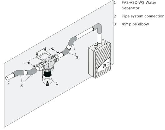
Installing the FAS-ASD-WS Water Separator in the pipe system
