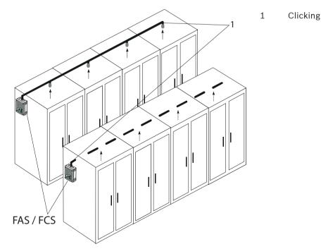
Principle of equipment monitoring with FAS-420 series aspirating smoke detectors
