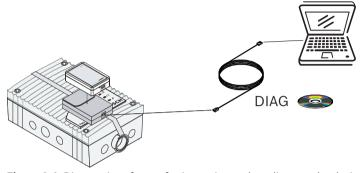
**Figure 3.4:** Diagnostic software for importing and reading out the device data The FAS-ASD-DIAG Diagnostic Software enables the saved and current statuses of the FAS-420 and error messages to be saved on a PC or laptop.
