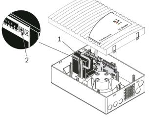
Air-pressure-independent calibration of the airflow sensor
