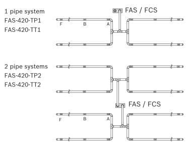
Double U-pipe system for space protection
