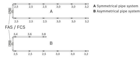
Tab. 4.1: Example of a symmetrical and an asymmetrical U-pipe system
