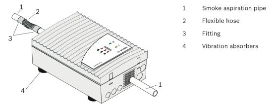
Absorption of the operating noises caused by airflows
