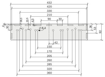
Figure 5.3: Bore distances with mounting type MT-1
