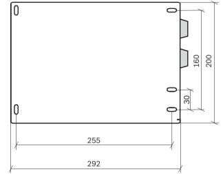
Figure 5.2: Bore distances of FAS-420 without mounting
