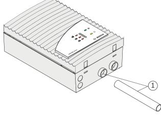
Connecting the aspiration pipe to the FAS-420 Aspirating Smoke Detector
