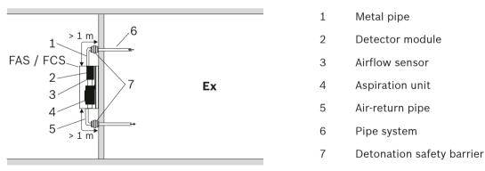
Detonation safety barrier in the aspiration pipe system and if necessary in the air-return pipe
