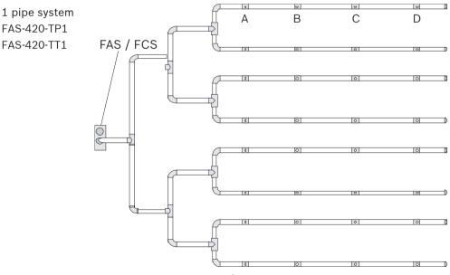
Quadruple U-pipe system for space protection
