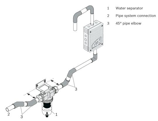
FAS-ASD-WS Water Separator for condensing water vapor and collecting condensate from the pipe system
