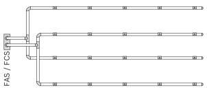
Pipe configurations for dual detector dependency
