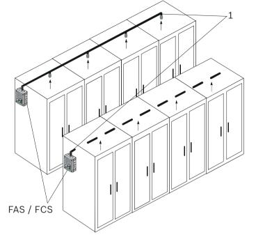
Principle of equipment monitoring with FAS-420 series Aspirating Smoke Detectors
