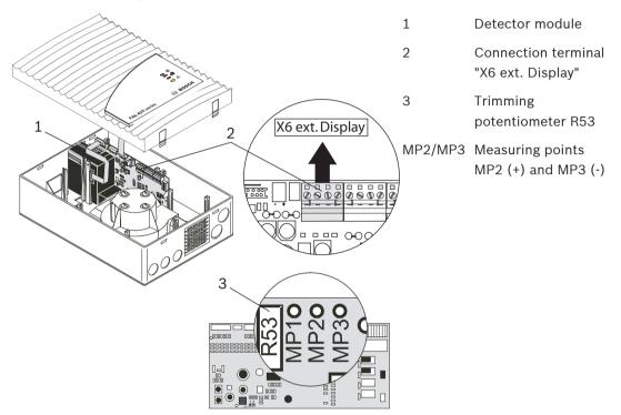
Air-pressure-dependent calibration of the airflow sensor
