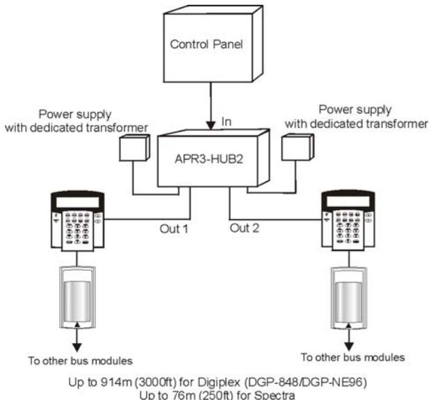
**Figure 2: Connecting the APR3-HUB2**
