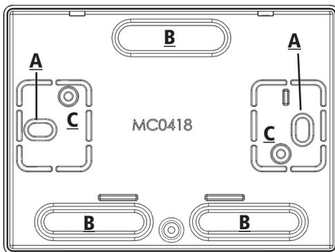
Knock out (where necessary) the points B, for cable entry.
