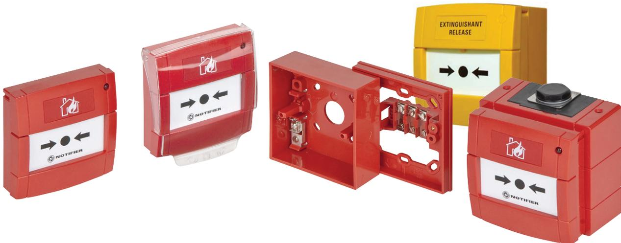
The MCP1A-R470 range are manual call points, both with a 470 Ohm resistor and Normally Open contact, complete with glass. The MCP1A-R470FG-01 is designed for semi-flush mounting and the MCP1A-R470SG-01 is designed for surface mounting. The call points are designed to provide a manual alarm interface to non addressable fire alarm control panels. Both call points are supplied in the standard red colour.
