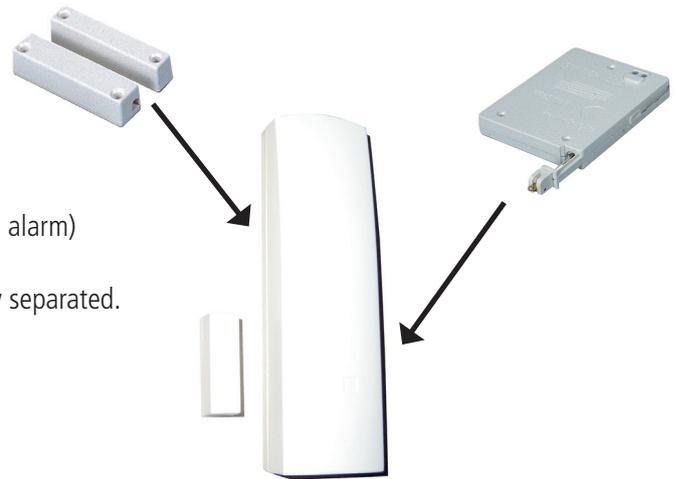
**CU800** is a bidirectional wireless device with 3 inputs entirely separated.
