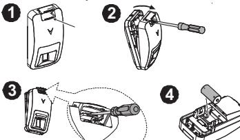
1. On the indicated location, lift the screw cover upward using your thumb.
