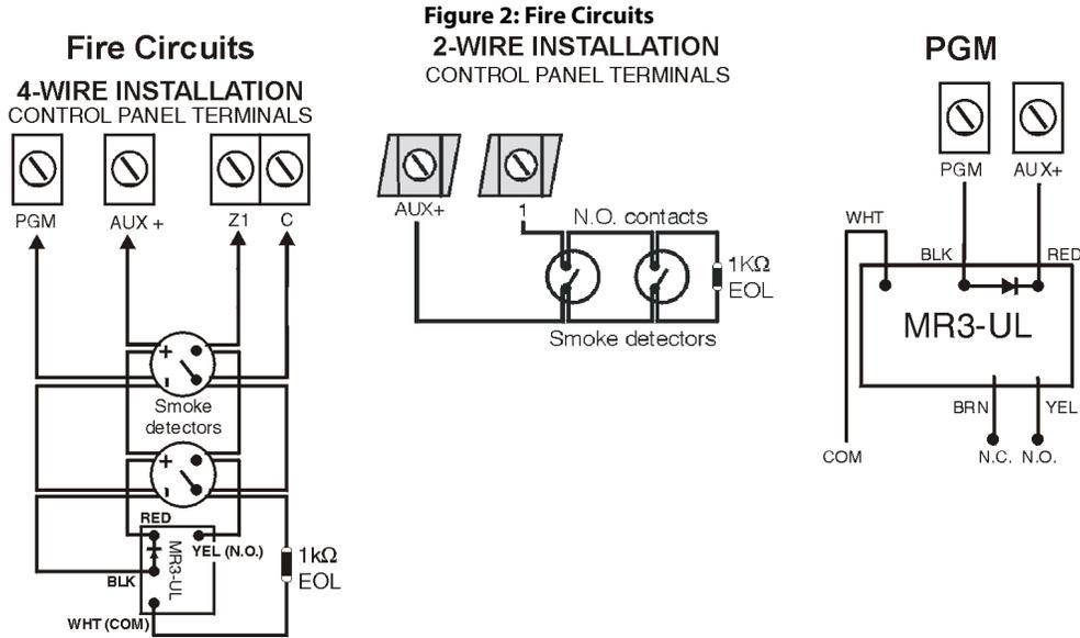
**Figure 2: Fire Circuits**
