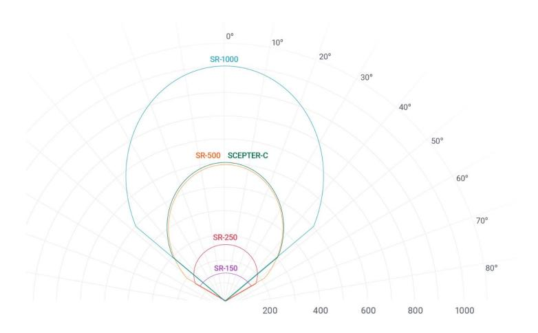
Figure 6: SR-Series Maximum Coverage Diagram (Top View)
