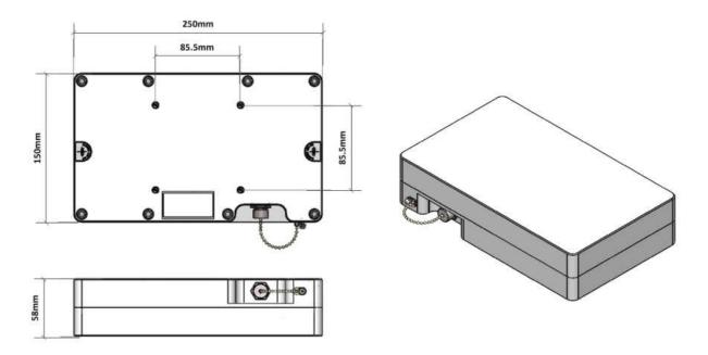
Figure 4: SR-500F/SR-500I/SR-250F/SR-150F Mechanical Dimensions and Mounting Holes
