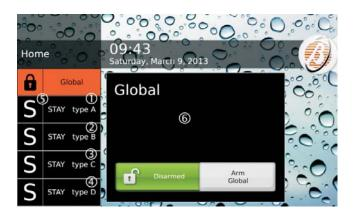
**Figure 27** Arming by the Touch Keypad: labels **1**, **2**, **3** and **4** can be customised, as explained in the text; the corresponding Special arming initial letter will be put in position **5**; the description assigned to the arming selected will appear in window **6**, as explained in the text.
