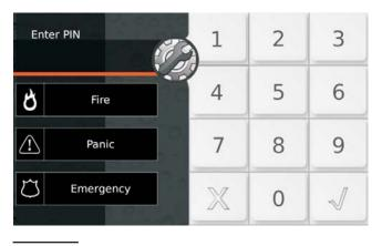
Figure 25 Default labels of the Super Keys on the Touchscreen Keypad.
