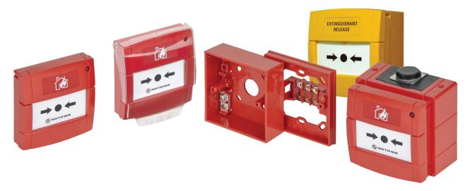
The MCP1A-R470 range are manual call points, both with a 470 Ohm resistor and Normally Open contact, complete with glass. The MCP1A-R470FG-01 is designed for semi-flush mounting and the MCP1A-R470SG-01 is designed for surface mounting. The call points are designed to provide a manual alarm interface to non addressable fire alarm control panels. Both call points are supplied in the standard red colour.
