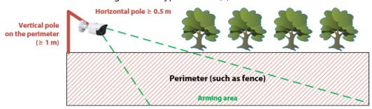
• When there are obstructions (such as trees and vegetation) around the perimeter, and wire netting on the perimeter, install a vertical pole separately. Keep the pole 1 m from the perimeter, and 1 m higher than the perimeter (installation height 3 m-5 m).
