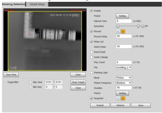
Step 3 (Optional) Select Max Size or Min Size, click Draw Target, and then drag the corners of filter box to make the box larger or smaller.
