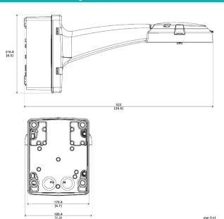
These units can be mounted directly to a wall or other flat surface. Optional pole and corner mounting accessories are also available, allowing you
