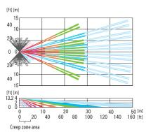
The detection angle of the creep zone can be adjusted  $\pm 135^{\circ} horizontally$  as shown in gray.
