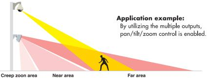
Note: The ambient temperature, installation height and mounting angle may change the detection ranges for each of the areas.
