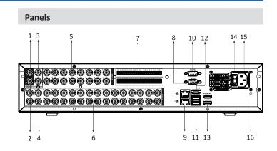
1 Audio Out 2 Video Out 3 Mic In 4 Mic Out 5 Audio In 6 Video In 7 Alarm Input/Output 8 VGA Port 9 Network Ports 10 RS-232 Port 11 USB Ports 12 eSATA Port 13 HDMI Ports 14 Power Switch 16 Ground 15 Power Input
